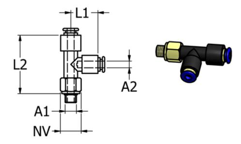
Ext. hose diameter A2 = 3 mm L1 = 12 L2 = 28.5 NV = 10 Thread A1 = M6
